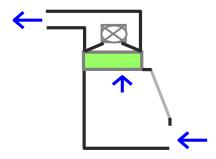
The filtered air is normally discharged into the atmosphere but in exceptional circumstances it is possible to recycle the air in the laboratory provided it has been passed through two HEPA filters and the procedure has HSE approval.
