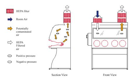
**NOTE:** Microbiological safety cabinets should not be confused with other **laminar flow** cabinets, in particular with horizontal laminar outflow cabinets which direct air towards the operator. Laminar flow cabinets must not be used for handling infectious, toxic or sensitising materials.
