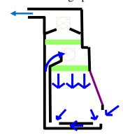
The air flow around the front of a Class 2 cabinet is very delicately balanced and easily disturbed and thus if the cabinet is badly sited and/or set up, it may not provide the protection required.
